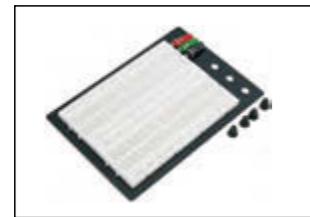
ITEM:EB04B-2S4P 1680 tie-point 4 Power lanes,400 PTS 2 Standard double-strips,1280PTS SIZE:17.12×12.84×0.83 cm
