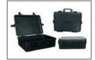
ITEM:EPC021 Material:ABS/PP I D:L565×W410×H193 mm OD:L632×W474×H212 mm Weight:5900 g
