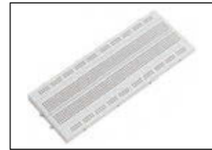
ITEM:EB04 840 tie-point 2 Power lanes,200 PTS 1 Standard double-strip,640 PTS SIZE:17.12×6.42×0.83 cm
